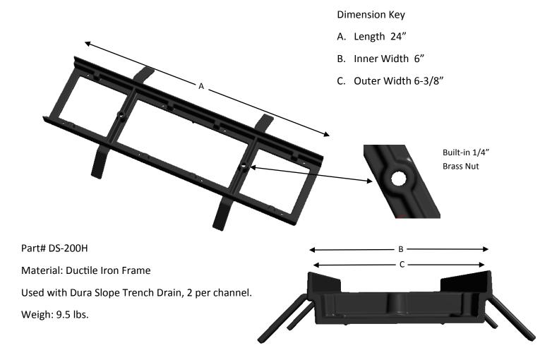
Dura Slope Ductile Iron Frame provides a Class D load rating of 326-575 psi and is suitable for heavy-duty hard tire equipment at speeds less than 20 mph. The DS-200 Ductile Iron Frame is recommended for use with pneumatic tire traffic such as fork lifts. The ductile iron frame can be used with the cast and ductile iron grates.
